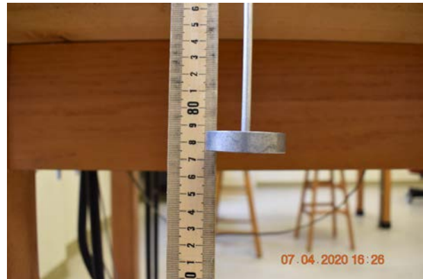
Figure 4 Measurement of drop height
